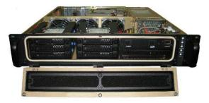
This system is packed in a 2U 20.1 inch depth aluminum chassis with a ¼ inch front panel for improved rigidity and ruggedness. This system is designed with high speed data recording through the use of rotating or solid state drives (SSD) disks. This rugged solution provides up to 12 Terabytes (TB) of storage capacity with rotating drives or 7.2 TB with solid state drives.
