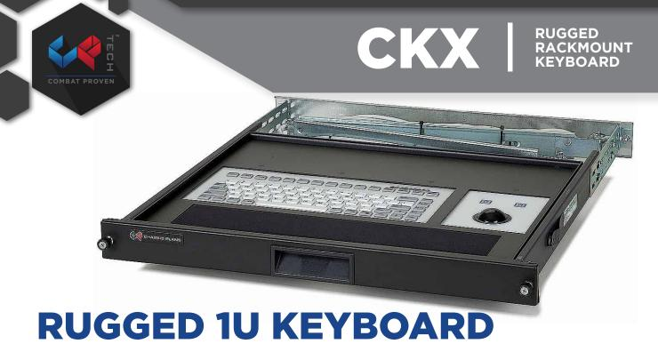
Our CKX Keyboard can be used for many rugged military applications. You have the option of a trackball or touch pad. The keyboard has exceptional strength, is low weight, and works well under extreme temperature swings. The drawer includes friction slides for mounting into a 19" rack. The drawer uses screw locks to secure it into the rack for transportation.
